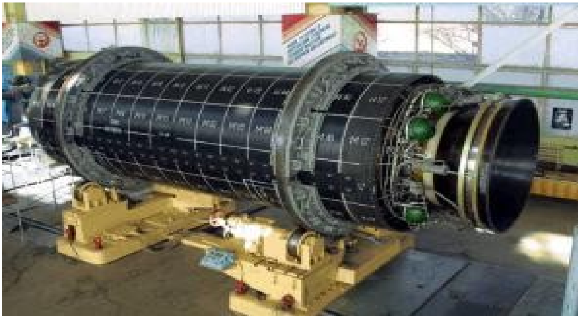
15D305 solid motor for RT-23 ICBM
