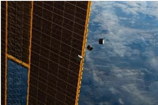
Cubesat deploy from ISS, 2012
